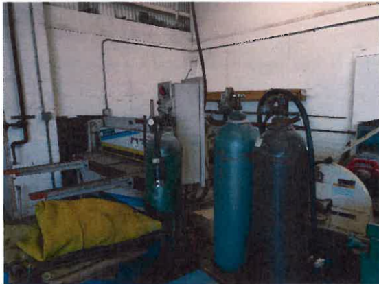
Figure 11: Unsecured large equipment.
